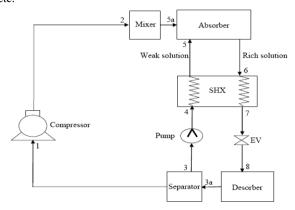
**Fig.1** Schematic Diagram Of Vapor Compression-Absorption Refrigeration System [10]
