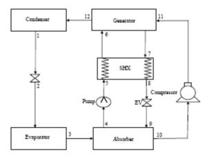
**Fig.4** Schematic Diagram Of Vapor Compression-Absorption Combined Or Hybrid Refrigeration System [41]
