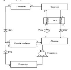
**Fig. 2** Schematic Diagram Of Vapor Compression-Absorption Cascaded Refrigeration System In Series Configuration [23]
